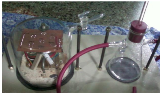
Fig. (3) Glass Gas Chamber
