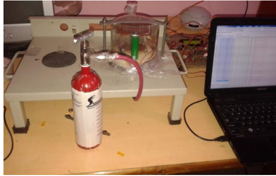
Fig. (5) Hardware setup Gas identification unit
